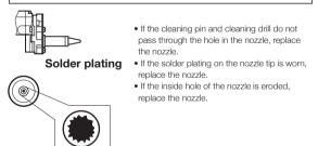
Hole is damaged by erosion.
