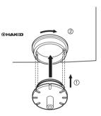
3. After replacing the ceramic paper filter, press the filter case cover with its tabs inserted into the corresponding slots in the filter case then turn clockwise to lock it.
