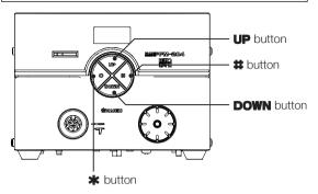
The front panel of the HAKKO FM-204 has four controls.
